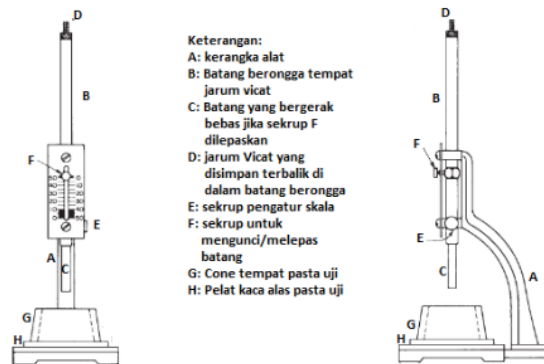
Gambar 1. Skema Alat Vicat (ASTM C 187)
